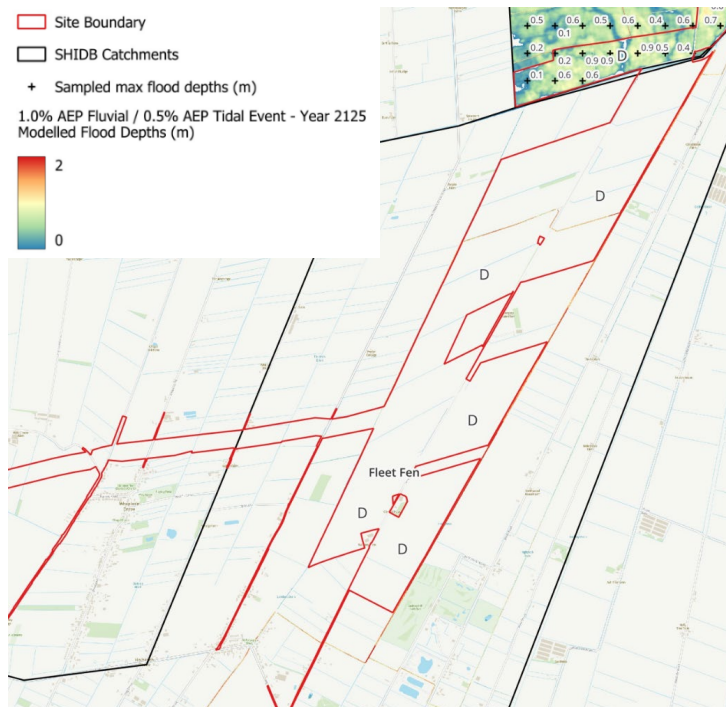
Plate 5-9: 1% AEP plus 13% climate change Pump On Scenario flood extents in the Fleet Fen Catchment
